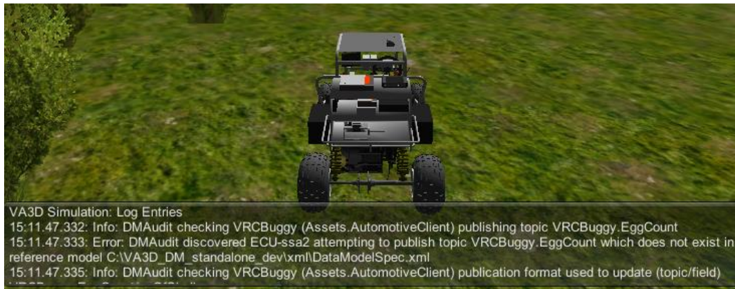
Figure 9: Screenshot Showing Dmaudit Tool Reporting Publication to a Topic in Contravention of The Reference Model.
